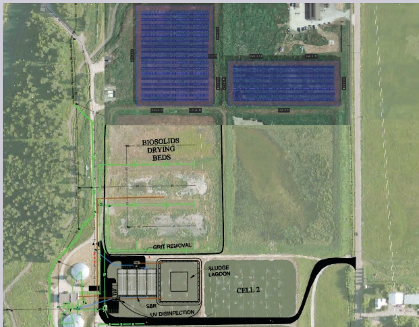
FIGURE 4. POSSIBLE SITE DESIGN OF NEW WHITEFISH WASTEWATER TREATMENT PLANT. Showing proposed 1.7 MW solar farm (blue). Courtesy Anderson-Montgomery Consulting Engineers and Aeon Renewable Energy.
