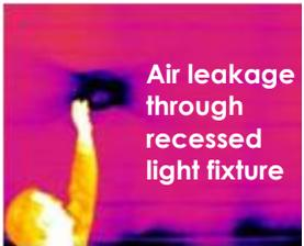
An infrared (IR) camera shows the temperature of the house's surfaces. Improperly insulated areas will appear colder than expected in winter and warmer than expected in summer. Consider having an IR investigation to confirm the house has been properly insulated. An IR investigation conducted with a blower door analysis can detect air leakage.
